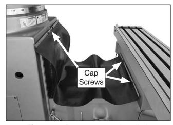
Figure 13. Rear way cover installed.
